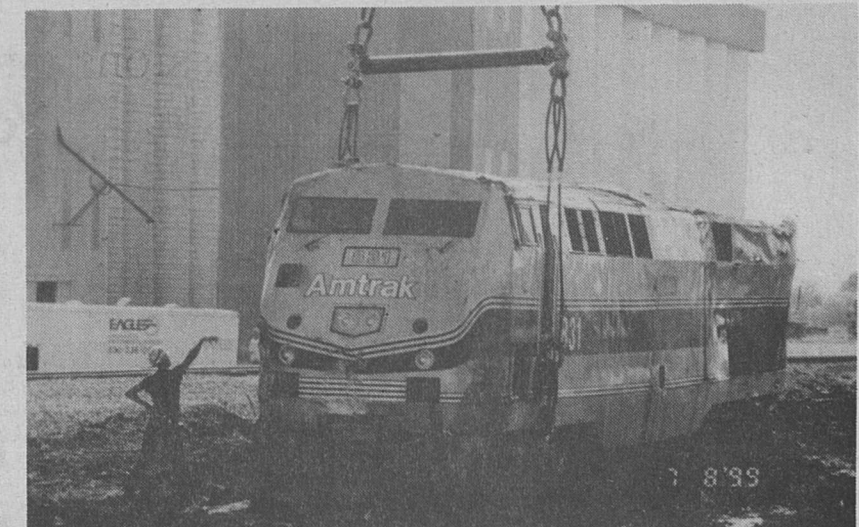
Cleaning up the derailment site and repairing the rails went on through Thursday night into Friday. Here a worker is directing the crane as it lifts the engine into an upright position to be loaded on a trailer.
