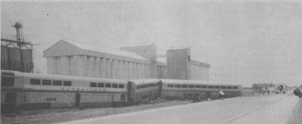
Approaching the front of the train on Hwy. 90-A, one could see that most of the completely derailed cars were in the forward section. The remaining cars more or less "jumped" the tracks.
